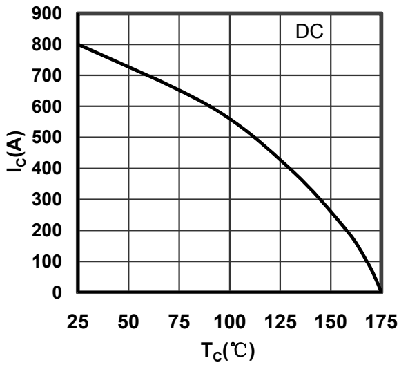
Figure 7. Collector Current vs Case temperature IGBT -inverter
